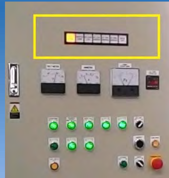
ERROR INDICATOR: Light up error reason
